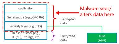
Data in execution can be protected by Trusted Execution Environments (TEEs) such as Intel SGX, ARM TrustZone, and SecureElements. TEE hardware enforces three guarantees:
